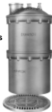
Figure 1. 36" Diameter Tower Sections
