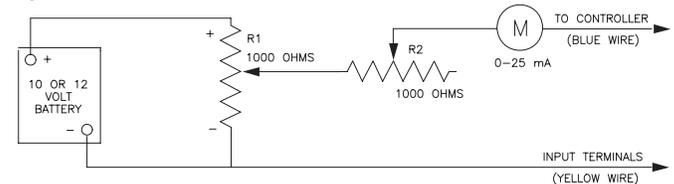
Test Unit for milliamp Input Positioner – Set R1 all the way toward the plus end. Adjust R2 for a 20 mA reading. Varying R1 will now provide input signals between 4 and 20 milliamps.
