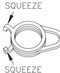
Squeezing together the two small protrusions from the cam, as shown above, loosens the spring and allows adjustment. Needle nose pliers may prove to be helpful when installing the cams, but are not required.
