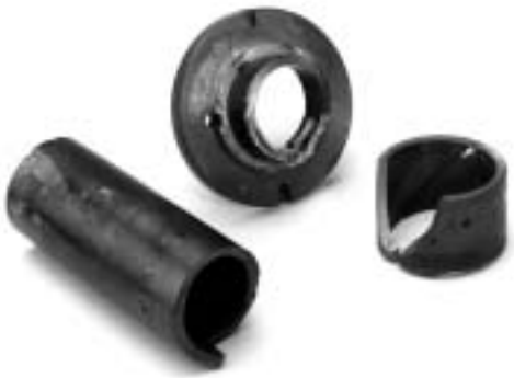
Figure 2: Failed Bushing and Journal Parts Caused by Dry-Run
