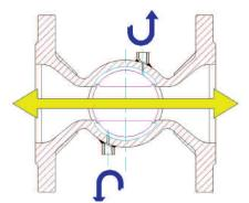
When valve is in fully closed position, side ports open to allow passage of a monitoring gas through plug waterway to verify the position. In any other plug position, the side ports remain blocked.
