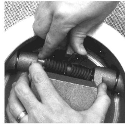
Fig. 5 Installation of Auxiliary Spring Assembly
