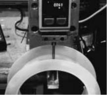
The top photo shows a Durco PTFE liner while the bottom photo shows a competitive PFA liner. It can be easily observed that the Durco liner is almost twice as thick and, thus, is more permeation resistant.
