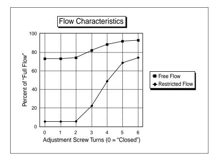
To determine the flow for a specific application, look up the maximum flow for the spool valve size and supply pressure from Bulletin PS0006-CV. Multiply the valve by the percentage shown in the above graph for the specific adjustment setting. For example, for a high flow spool at 60 psi and 4 turns adjustment, the restrictive flow will be  $0.49 \times 17.5 = 8.6$ . The free flow will be  $0.88 \times 17.5 = 15.4$ .
