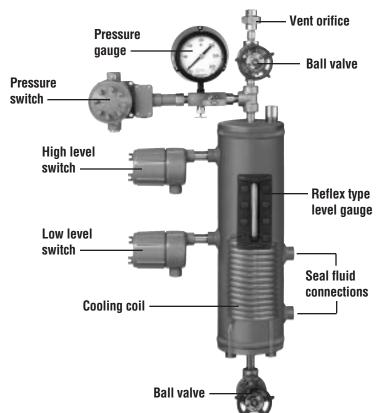
An advantage of a closed-loop supply tank system is its ability to indicate the condition of inner seal leakage based on the fluid level measurements over a set period of time. Optional level monitoring devices are available for early detection of either high or low liquid levels and pending seal failure.
