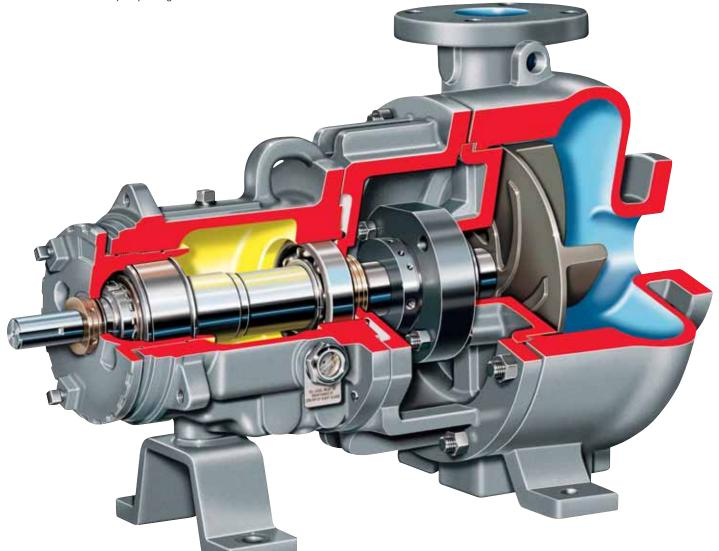
*Vortex Action* minimizes abrasive wear while maintaining solids integrity because only a fraction of the media contacts the impeller
