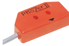
Type P / PP Phazer II (2) SPDT Proximity 3 amp @ 120 VAC, 2 amp @ 24 VDC, 100 Watt Max. Minimum 50 mA
