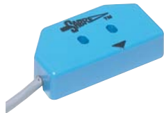
Type E / P1 Sabre Switch (2) SPDT Proximity 1 amp @ 120 VAC, 1 amp @ 24 VDC, 25 Watt Max. Minimum 1 mA
