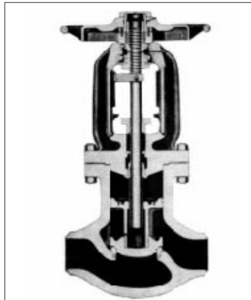
Figure 1: Large cast-steel valve with bolted-bonnet design, from Edward Catalog No. 103, June 1949.
