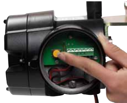
Press button and APEX 9200 will auto calibrate itself.
