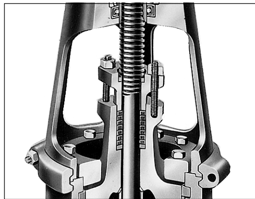
Figure 13: A bronze bushing protects against stem damage due to gland cocking.
