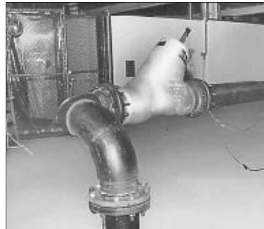
Figure 3: Another example flow disturbance test installation with two upstream elbows, this time employed with a size 10, Class 1500, Flite-Flow® inclined-bonnet piston-lift check valve.
