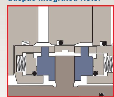
A ductile rotor/sleeve dry gas seal reduces the risk of brittle rotating seal face failure and the associated consequential effects to the equipment. The ductile rotor design is commonly used in high speed gear compressors and turbo-expander applications as well as in machines having a limited seal cavity area.
