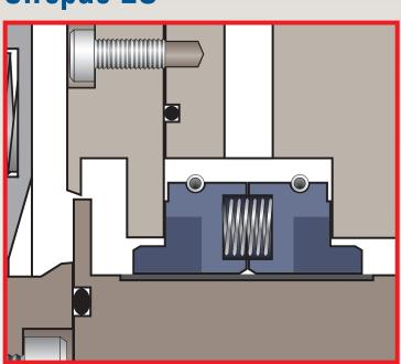
Engineered segmented carbon ring that is a non-contacting lift-off design with minimized clearances for low gas consumption and allows for same gas consumption under static and dynamic conditions.
