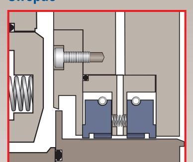
Non-contacting, bi-directional segmented carbon rings protect the dry gas seal from oil contamination.
