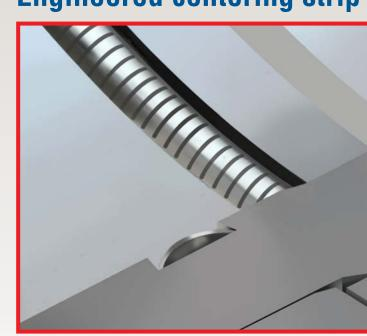
Used on seals that exceed the size and speed permitted for o-rings to center the sleeve on the shaft. The centering strip is fully captured in a dovetail groove.
