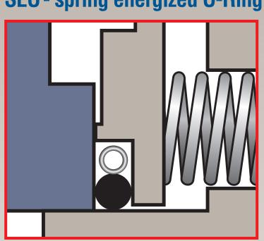
LoDrag<sup>™</sup> secondary dynamic seal provides radial compression to seal the gas medium. Live loading of the dynamic o-ring reduces slip-stick hang-up.
