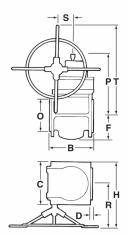
Flanged valves have face-to-face dimensions conforming to BS 5158 PN 10/16 & BS 2080 Class 150 Short, ANSI B16.10 & API 6D Class 150 Short. These valves are thus interchangeable with equivalent gate valves. Flanged valves have patterns conforming to BS 5353, BS 5158, ANSI B16.34, API 6D & API 599 Short (with steel plug).
