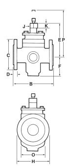
Valves have face-to-face dimensions conforming to BS 5158 PN 10/16, BS 2080 Class 150 Short, ANSI B16.10 & API 6D Class 150 Short. These valves are thus interchangeable with equivalent gate valves. Valves have Patterns conforming to BS 5353, BS 5158, API 6D & API 599 Short (with steel plug).
