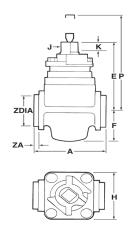
Flanged valves have face-to-face dimensions conforming to BS 5158 PN 10/16 & BS 2080 Class 150 Short, ANSI B16.10 & API 6D Class 150 Short. These valves are thus interchangeable with equivalent gate valves. Flanged valves have patterns conforming to BS 5353, BS 5158, ANSI B16.34, API 6D & API 599 Short (with steel plug).
