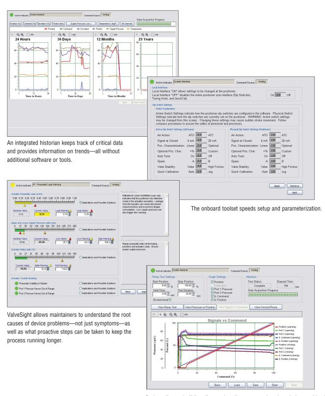
Both on-line and off-line diagnostics allow users to benchmark the combined performance of valve, actuator, positioner and control signal. Current performance can be compared to stored values as well as the original factory "birth certificate."
