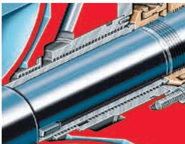
**Serrated sealing bushings**
