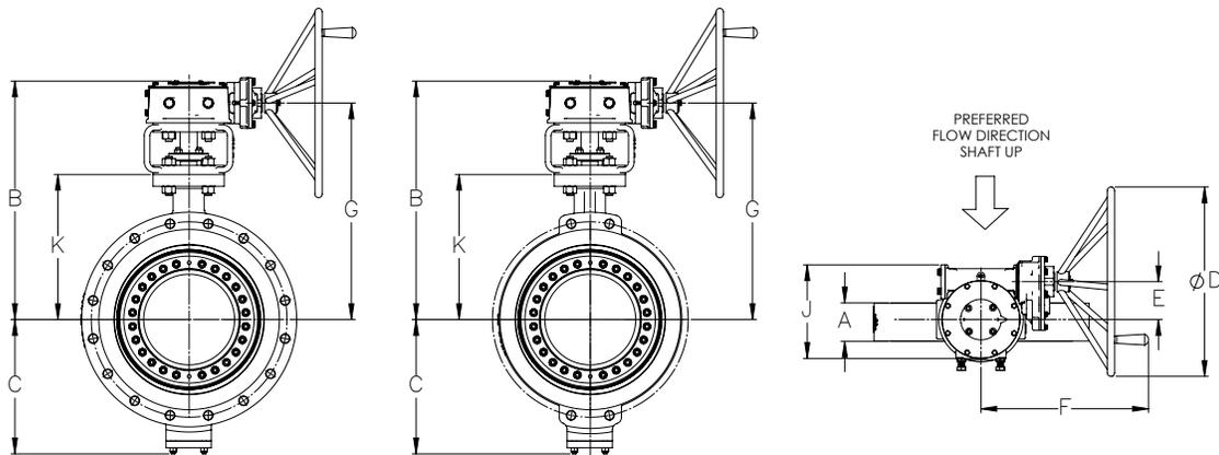
**Notes:** Flange dimensions per B16.5. Some sizes have tapped holes around the shaft area (top and bottom); consult factory for actual dimensions. Consult factory for pressure classes 900 and 1,500.
