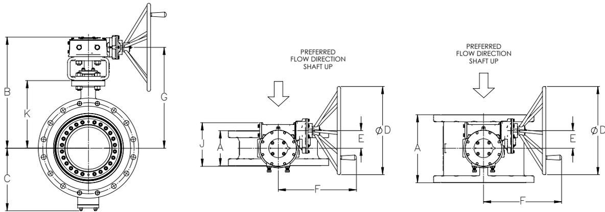
**Notes:** Flange dimensions per B16.5. Some sizes have tapped holes around the shaft area (top and bottom); consult factory for actual dimensions. Consult factory for pressure classes 900 and 1,500.
