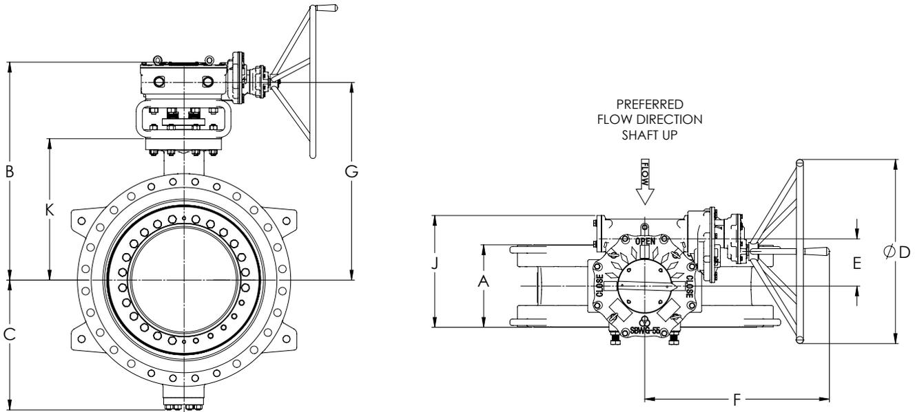
**Notes:** Flange dimensions per B16.47. Some sizes have tapped holes around the shaft area (top and bottom); consult factory for actual dimensions.
