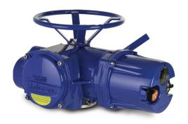
The MX can be directly mounted to any rising or non-rising stem valve. When combined with a Limitorque WG or HBC series worm gearbox, it can be used to control butterfly, ball and plug valves, as well as damper drives, flop gates or similar devices. MX actuators can also be coupled with Limitorque V series bevel gearboxes or SR series spur gearboxes for motorized operation of multi-turn valves when extended operating times or reduced motor current requirements are required.
