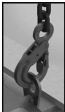
Figure 1a: Use of Lifting Lug on the housing
