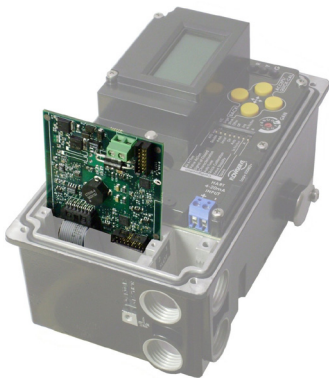
Auxiliary Card Being Installed
