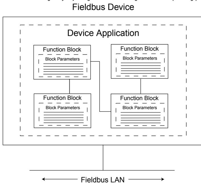
**Figure 1.5 Fieldbus Devices Contain Device Applications and Function**
