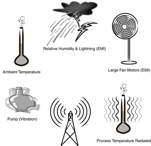
**Figure 4.1 Typical Mounting Area Considerations Prior to Installation**
