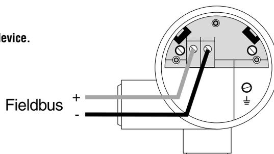
4. At the junction block, connect a fieldbus terminator in parallel with the device.
