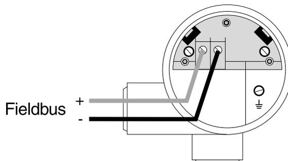
**Figure 5.5 Logix 3400IQ Digital Positioner Terminal Block**
