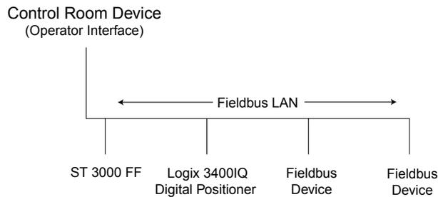
Figure 1.4 Fieldbus Connecting Control Room and Field Devices
