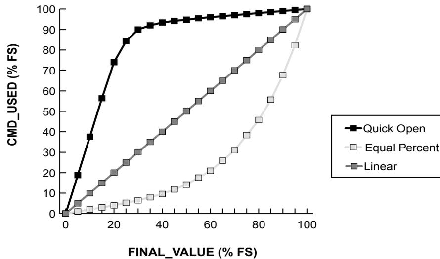
Figure 10.3 Logix 3400IQ Digital Positioner Characteristic Curves
