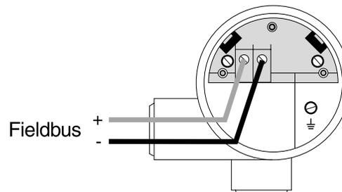
**Figure 5.6 Logix 3400IQ Digital Positioner Terminal Block**
