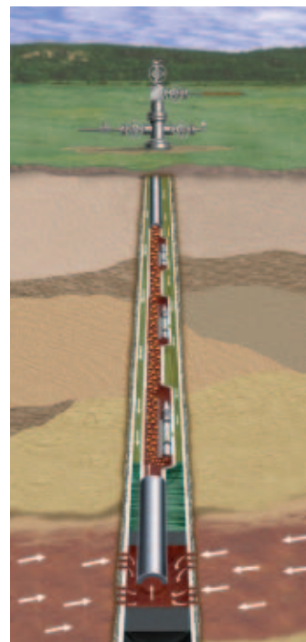
Figure 1. Formation pressure lifts the oil-water column and forces fluid out of the well bore.
