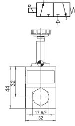
Port 3 (Exhaust) via M5 thread in top of Stem
