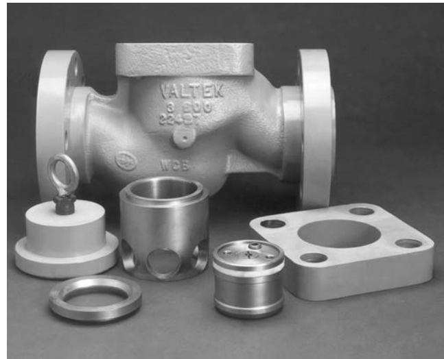
Shown above are the individual parts of the Tek-Check non-slam check valve: (from left to right) bonnet, seat-ring, retainer, piston, and bonnet flange. The interchangeable Valtek globe body is shown in the background.
