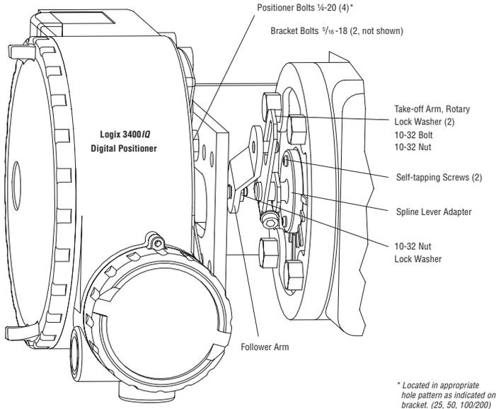
The standard rotary mounting applies to Valtek valve/actuator assemblies that do not have mounted volume tanks or handwheels. The standard mounting uses a linkage directly coupled to the valve shaft. This linkage has been designed to allow for minimal misalignment between the positioner and the actuator. The tools required for the following procedure are:
