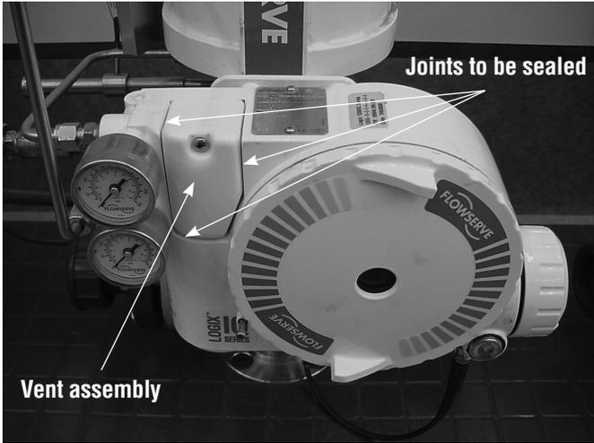
A small desiccant package as shown can be included under the sealing tape to insure proper protection.
