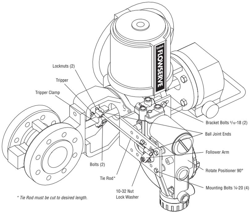
The optional rotary mounting applies to Valtek valve/actuator assemblies that are equipped with mounted volume tanks or handwheels. The optional mounting uses a four-bar linkage coupled to the valve shaft. The following tools are required:
