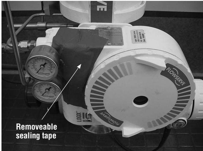
The sealing tape and desiccant should be removed when instrument air is permanently applied to the positioner.
