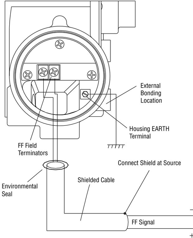
**C WARNING:** The green grounding screw must not be used to terminate signal shield wires.
