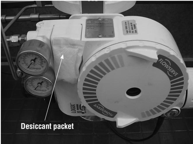
All of the edges around the vend assembly should be sealed similar to the picture below.
