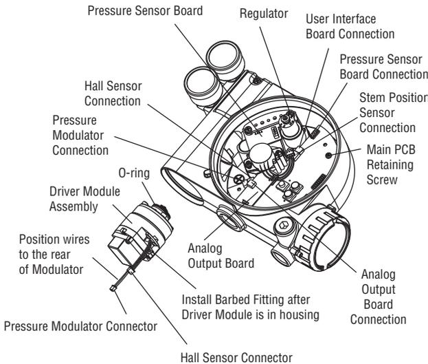
Figure 13: Spool Valve Cover Assembly
