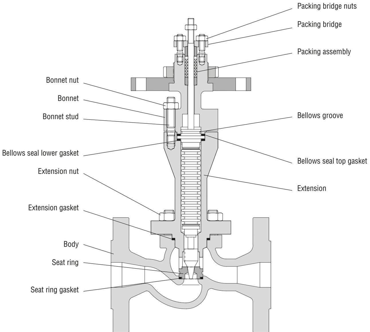
**Typical bellows seal valve configuration**
