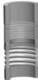
V-Ring packing live loaded
