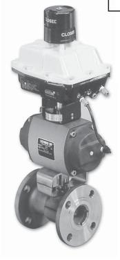
For applications involving moderate pressure drops and temperatures, Flowserve offers standard round port control valves in three-piece, wafer, and flanged valve body configurations. Standard seat material is Polyfill® with other resilient materials available. Shutoff is bubbletight. Control characteristic is equal percentage.
