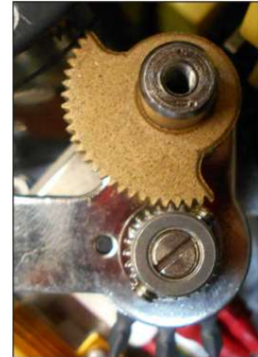
Figure 40: Alignment of the sector and potentiometer gear sets at the fully CW position (ref. only).
