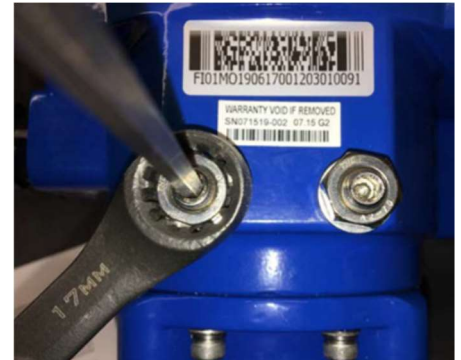
Figure 23: CCW mechanical stop
