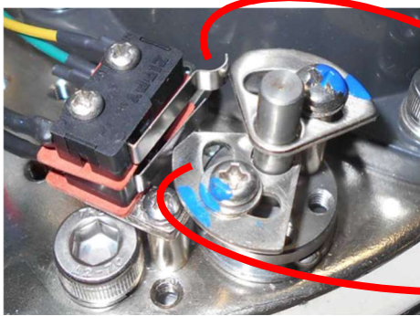
Figure 10: The torque switch cams and switches are shown in the normal operating position.
