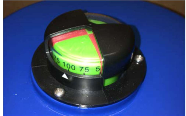
Figure 2: Red/green position indicator on top of actuator
