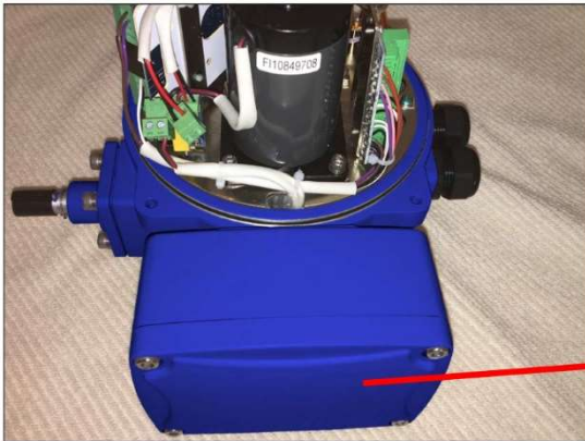
Battery and Controls Enclosure (No field terminations)
