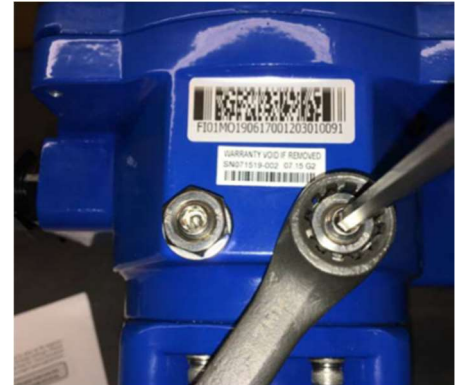
Figure 20: CW mechanical stop
