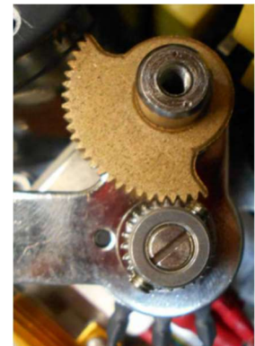
Figure 35: Alignment of the sector and potentiometer gear set at the fully CW position (see step 8).
