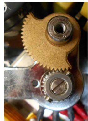
Figure 32: Alignment of the sector and potentiometer gear set at the fully CW position (see step 8).
