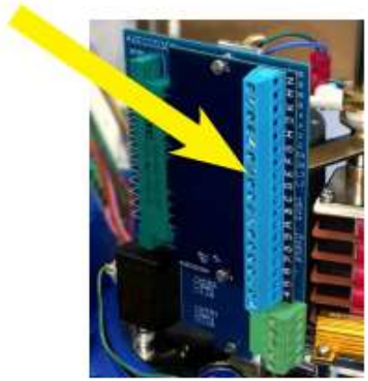
Figure 34: Proportional PCB details single-phase (120 – 230 VAC models)
