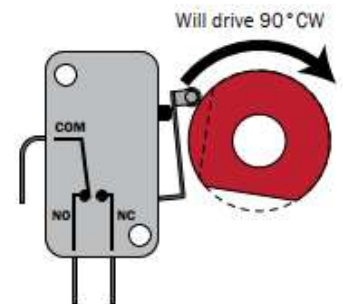
Figure 28: CW limit switch shown in the fully CCW position
