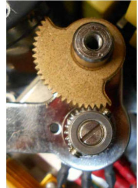
Figure 38: Alignment of the sector and potentiometer gear sets at the fully CW position (ref. only).
