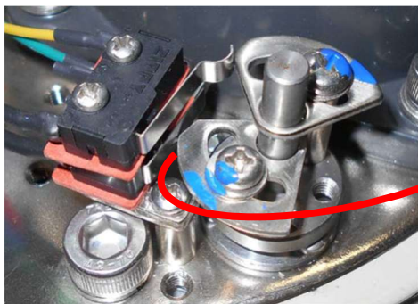
Figure 13: The lower cam is tripping the lower switch.
