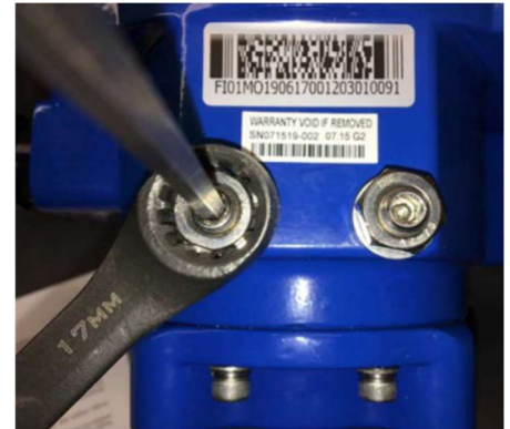
Figure 8: CCW mechanical stop
