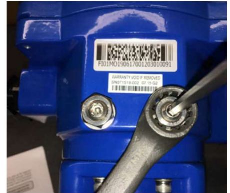
Figure 6: CW mechanical stop
