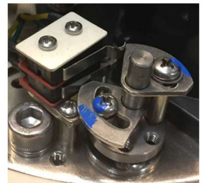
Figure 5: A torque switch (TS) is a secondary set of cams (switches) which further protects the actuator, equipment, and processes.
