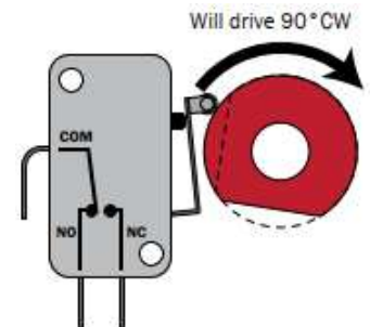
Figure 13: CW limit switch shown in the fully CCW position
