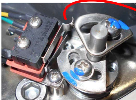
Figure 12: The upper cam is tripping the upper switch.
