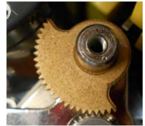
Figure 29: Alignment of the sector and potentiometer gear sets at the fully CW position (see step 8).
