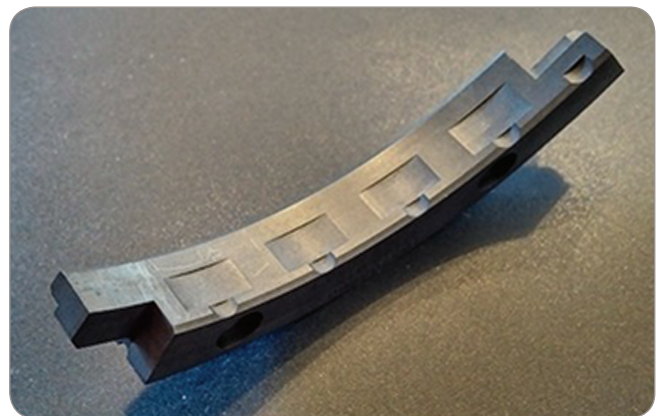
The T-grooves in this carbon ring segment allow gas to enter the seal gap and support ring lift-off, eliminating contact and wear.
