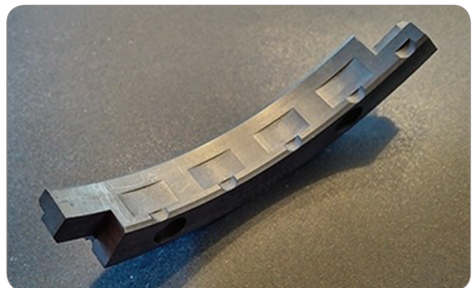
The T-grooves in this carbon ring segment allow gas to enter the seal gap and support ring lift-off, eliminating contact and wear.
