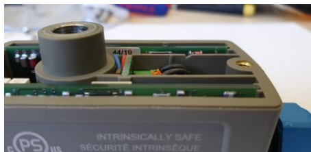
Figure 10: Cable inside of the housing
