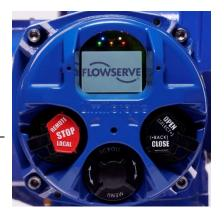
**Caution:** Do not use fasteners from MXa for securing the MXb control cover. The MXb flange on the control cover is thicker and requires a longer screw that is new to the MX product family. This new fastener is 45mm long and engages the housing 16mm after passing thru the 29mm flange on the MXb control cover.
