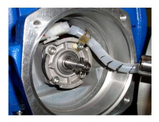
**CAUTION:** Ensure the grounding connector clip is pushed back to a minimum of parallel with relation to the worm shaft cap to prevent arcing to the stator.
