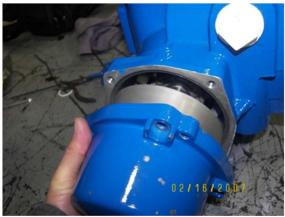
**NOTE:** If the motor sticks before fully engaging, remove and re-attempt installation insuring that the spigot remains straight.
