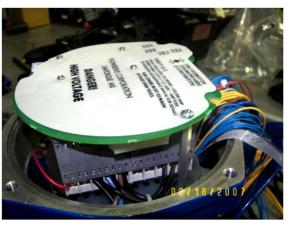
**CAUTION:** Ensure that the jumper on the power supply assembly is set in the correct voltage position.
