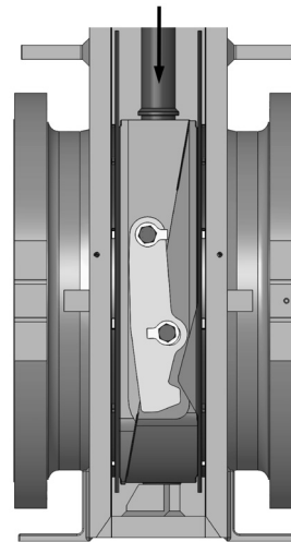
Figure 7a: Gate and segment expanded against seats
