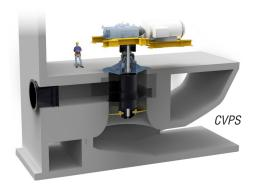
**Reduced construction time and costs.** Prefabricated elements, such as the suction bell and volute, significantly reduce on-site construction time and costs.
