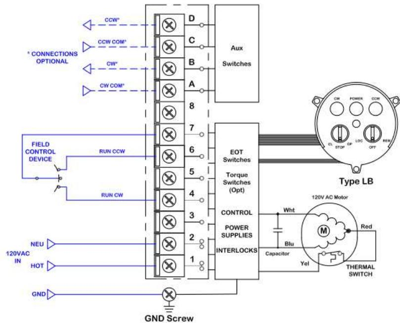
Figure 8: LB 120V wiring diagram shown, others similar
