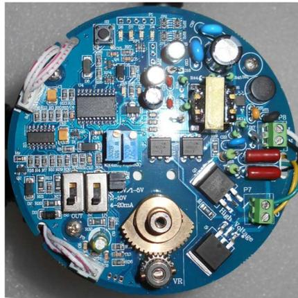
Figure 26: Actual proportional control board for 120 - 230 VAC models
