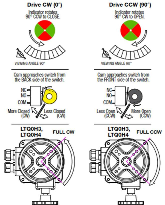
Figure 3: Examples of component rotations
