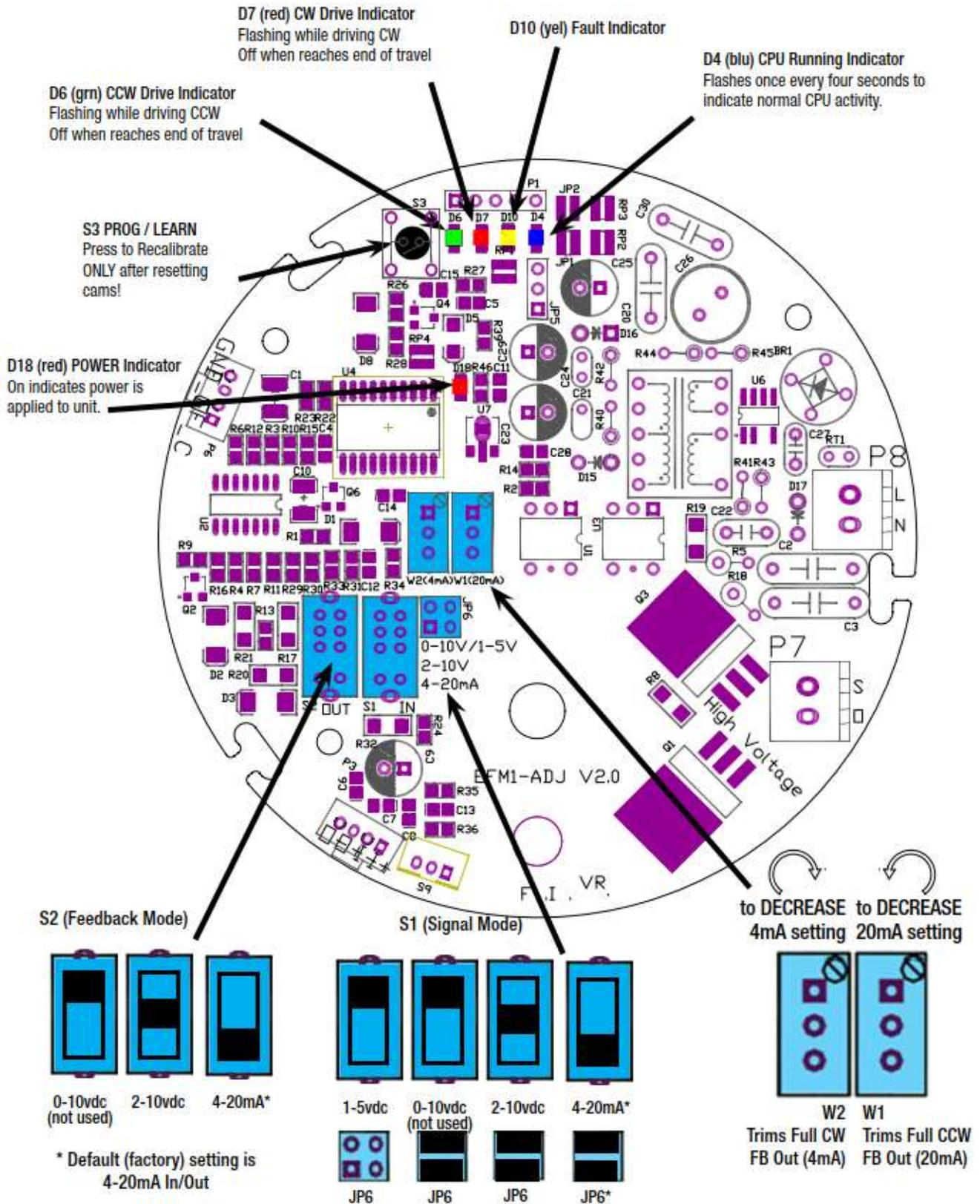
Figure 27: Proportional control board for 120 – 230 VAC models
