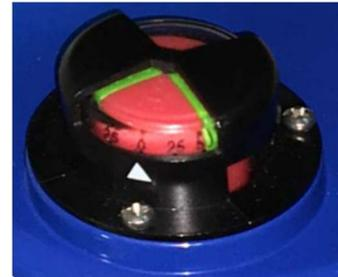
Figure 2: Red/green position indicator on top of actuator
