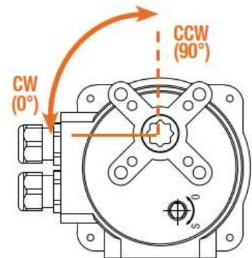
Figure 4: Note that the rotation seen from below is a mirror of the direction viewed from above
