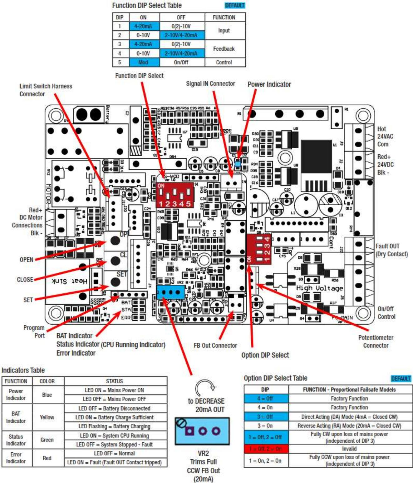
Figure 29: Proportional control board for 12 – 24 VAC/VDC models
