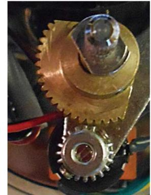
Figure 23: The correct alignment of the sector gear and pinion gear when the actuator is in its fully CCW position (CCW cam tripped)
