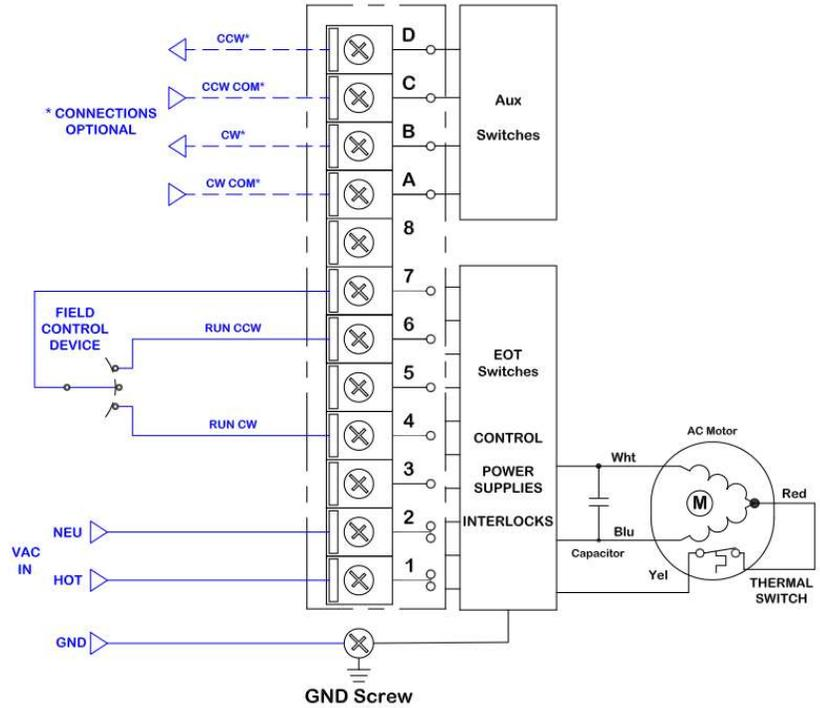
Figure 6: LB 120V wiring diagram shown, others similar
