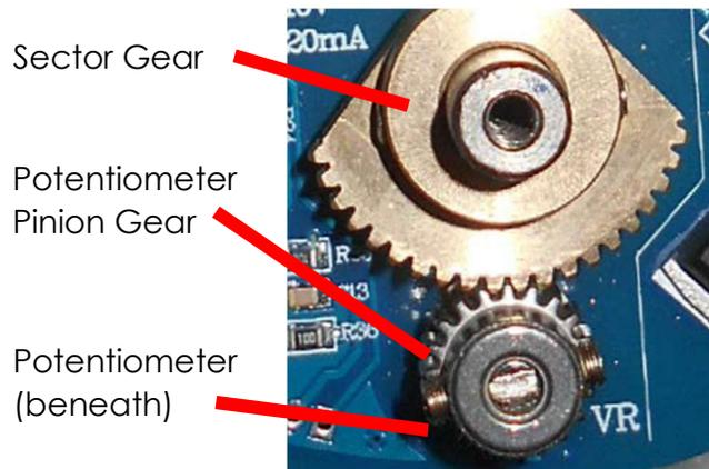
Figure 21: Proportional control sector gear / potentiometer pinion gear for 120 – 230 VAC models
