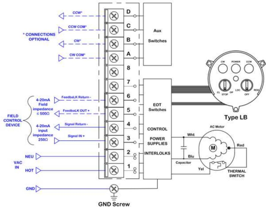
Figure 9: LB 120V wiring diagram shown, others similar
