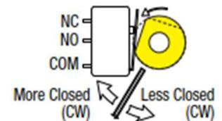
Figure 15: The cam approaches the switch from the back-side of the switch
