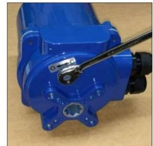
Figure25: Bottom mounted Manual Override
