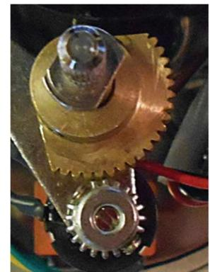
Figure 22: The correct alignment of the sector gear and pinion gear when the actuator is in its fully CW position (CW cam tripped)
