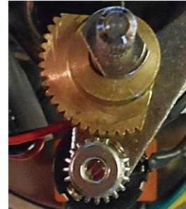
Figure28: Correct alignment of sector gear and pinion gear is critical to avoid damage to the position potentiometer (see Proportional Control Setup).
