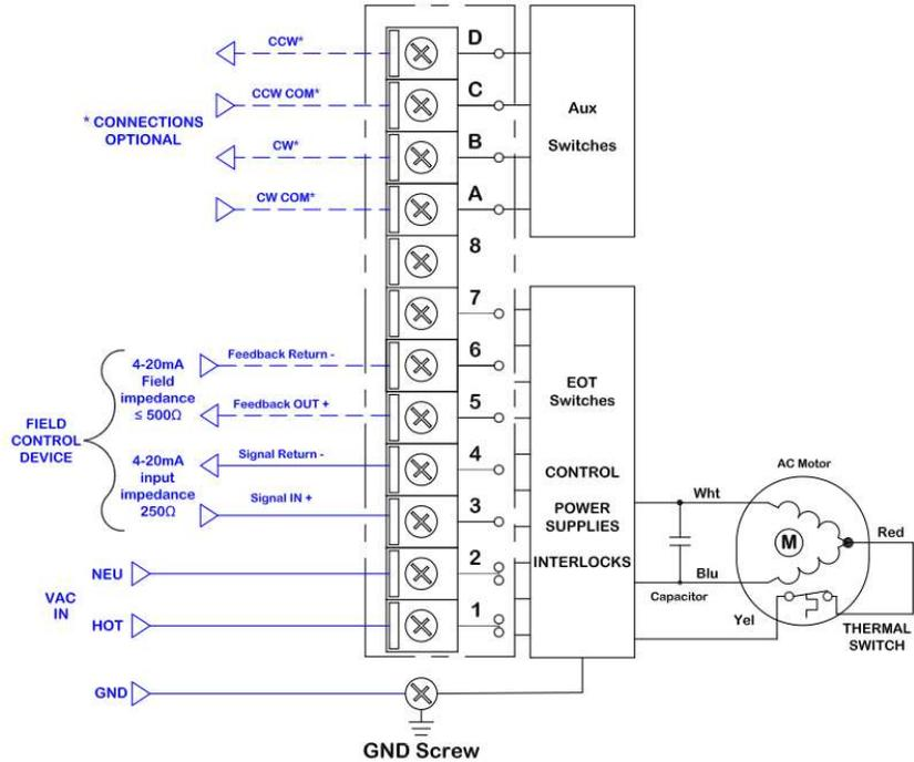
Figure 7: LB 120V wiring diagram shown, others similar
