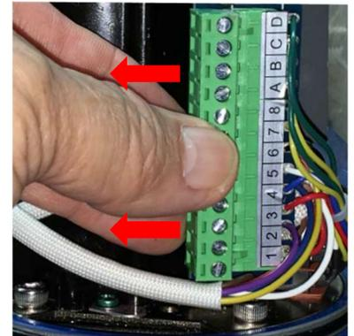
Figure 5: Removable terminal blocks facilitate field wiring and testing.
