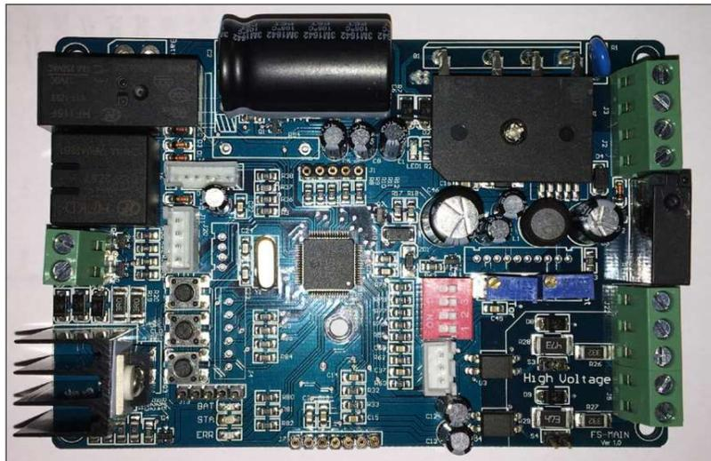
Figure 30: Battery Backup controller board for Open/Close applications
