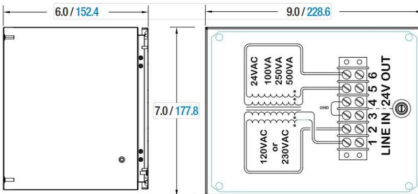
Figure 12: LTQ Series Transformer Enclosure Dimensional Data
