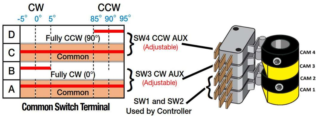
Figure 3: Auxiliary switch cam mapping
