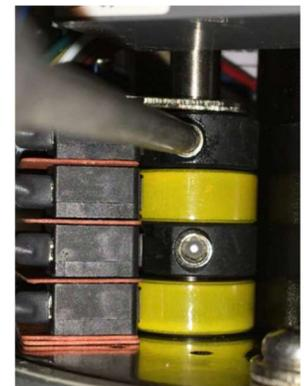
Figure 20: Cam 4 CCW auxiliary cam
