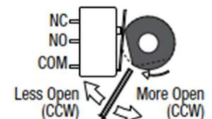
Figure 4: The cam approaches the switch from the front-side of the switch
