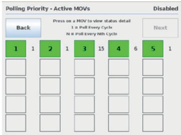
**Note:** to optimize the network efficiency, lower priority MOVs can be set to be polled at a user defined cycle.
