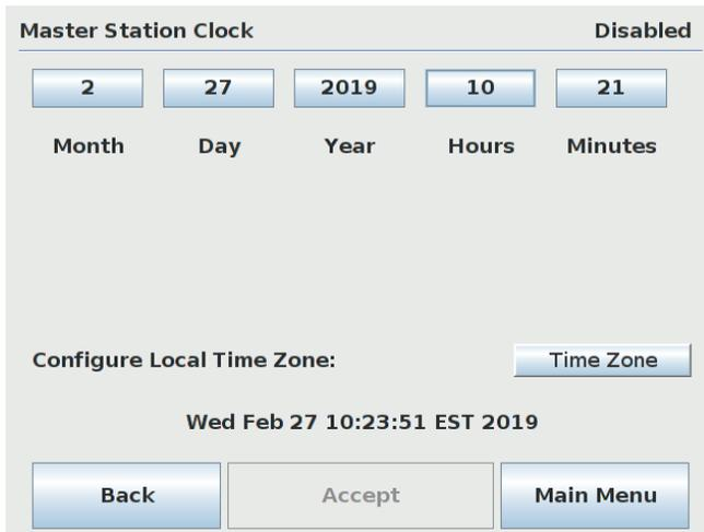
Additionally, the MSIV clock can be set to a specific time zone by selecting the Time Zone button in the Clock Setting Menu. The time zone is configured by selecting the region and locale in which the MSIV is located.
