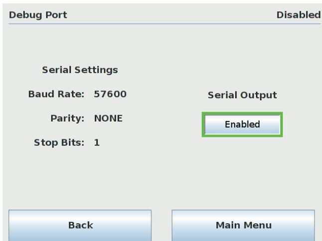
The Debug Serial port menu allows the user to enable/disable the serial debug port activity. When enabled, the debug serial port will transmit ASCII debug statements which can be monitored/logged via an external serial terminal. Static RS-232 serial settings are: Baud Rate = 57600, Parity = None, Stop Bits = 1. This port is configured as a standard RS-2323 DTE device. See section 4 Electrical Connections for serial port pinout details.
