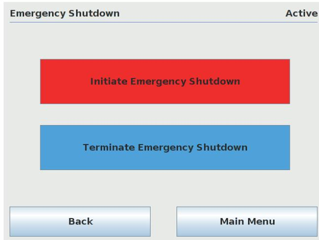
As shown in figure 6.4, two options are available: Initiate Emergency Shutdown and Terminate Emergency Shutdown. Once an emergency shutdown has completed and is no longer needed, the emergency shutdown state can be cleared by pressing the Clear Emergency Shutdown button.
