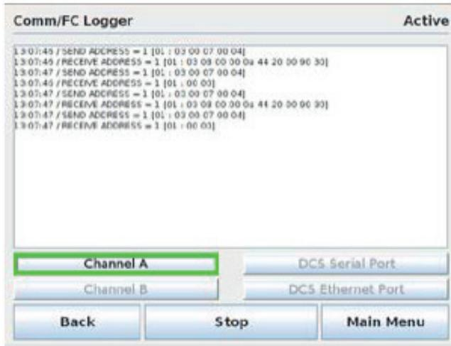
The Comm/FC logger captures Modbus requests and responses to/from the DCS and MOVs (channel A & B). The different communication channels can be enabled/disabled by pressing the corresponding buttons. Press “Start” to begin displaying communication activity on the screen. Press “Stop” to stop displaying communication activity on the screen.
