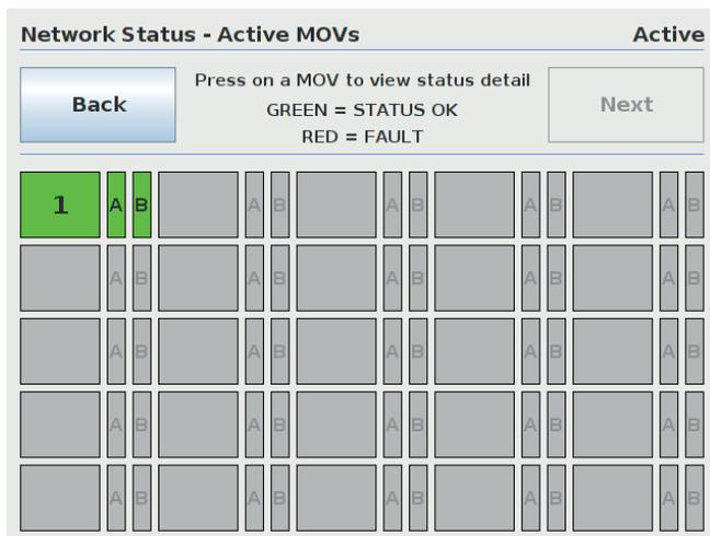
The numeric buttons represent addressed MOVs, while the A and B bars represent MOV communication channels A & B. The MOVs and their respective communication channels are constantly being monitored and will display green if OK and red if faulted. The user can advance to the MOV status screen by either touching an addressed MOV or touching the Back button to return to System Status screen, and then selecting MOV Status.
