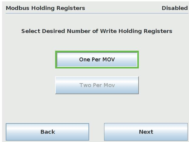
Selecting the “Next” button will advance the screen to a sample data table screen as shown below. Please note that a unique table is created starting at register 45001. Specific field unit registry convention is as follows: DCS Command Write Register = [(MOV address -1) \* (selected number of registers per MOV)] + 45001. Address affect is accounted for in the MSIV decoding process (i.e. 40,000).
