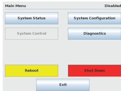
From here, the menu options are displayed based on the current user role. Each button represents a separate logical section of the Master Station.:
