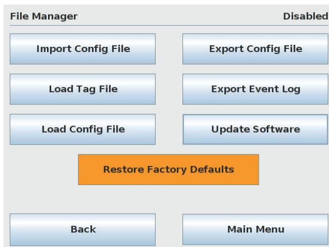
**Import Config File:** enables the user to import an existing system configuration file from a connected USB flash drive.
