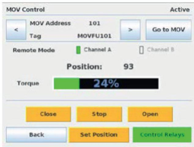
The Control Relays screen allows for a selected MOV's relay to be toggled on and off. To do this, the DCS function code 05/15 coils must be enabled. Additionally, the relays must be configured for network control within the specific MOV. Toggle a coil by tapping on the desired coil text box.
