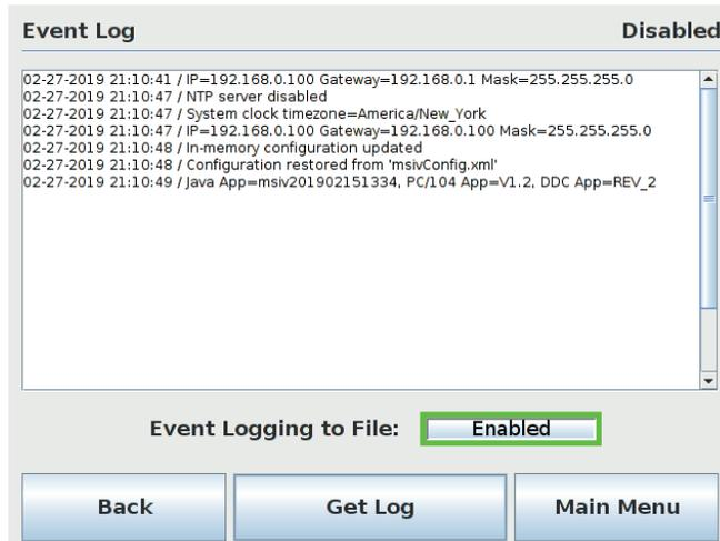
The Event Logger allows the user to display the last 20 events that were recorded. Every entry is defined, numbered, and time-stamped in order to maintain the logged data. Press the “Event Logging to File” button to Enable/Disable event logging. If event logging is Disabled, the MSIV performance may improve slightly, but Flowserve recommends enabling the event logging.
