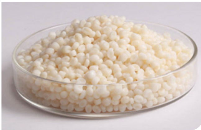
Polybutylene succinate (PBS) is a biodegradable plastic that can replace conventional hydrocarbon-based plastics for use in disposable tableware, paper cups and gas-barrier packaging for food.
