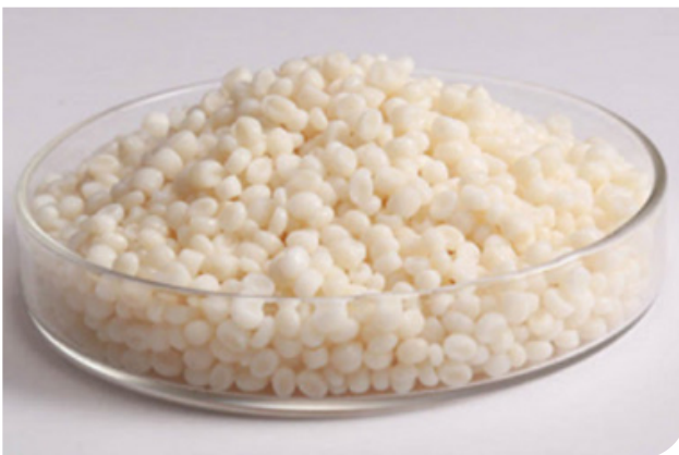
Polybutylene succinate (PBS) is a biodegradable plastic that can replace conventional hydrocarbon-based plastics for use in disposable tableware, paper cups and gas-barrier packaging for food.
