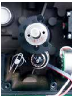
Potentiometer and cogwheel for 90° rotation
