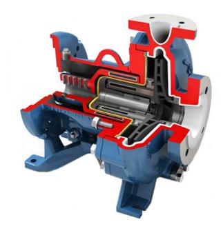
The INNOMAG TB-MAG pump all but eliminates the need for maintenance. There are no mechanical seal or ball bearings to fail, no shaft alignment or impeller adjustment needed, no emissions testing required, and no lube or oil to be changed.
