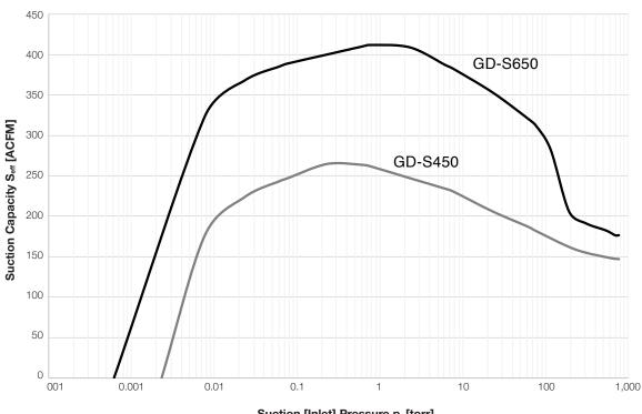
NOTE: Every operating point below the maximum characteristic curve is achievable by varying the speed.
