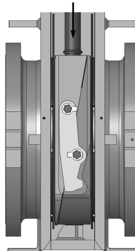
Figure 7a: Gate and segment expanded against seats
