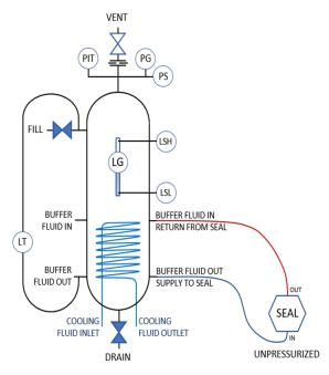
Figure 3: Recommended P&ID piping plan 52
