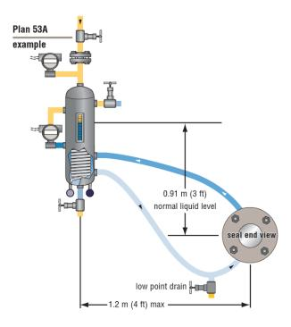
Figure 7: Piping Plan 53A mounting dimensions example
