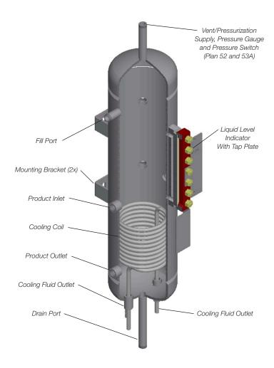
Figure 1: 682R51 Reservoir sectional view
