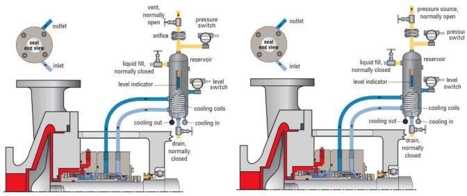
Figure 5: Piping Plan 52 configuration
