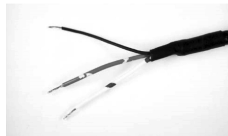
Figure 3.6 - Applying heat shrink tubing
