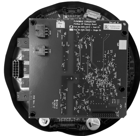
Figure 21 - MX/QX PB DP and Option Boards Mounted to MX/QX Main Board
