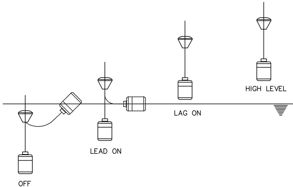
**Figure 4: Float Switch Installation**
