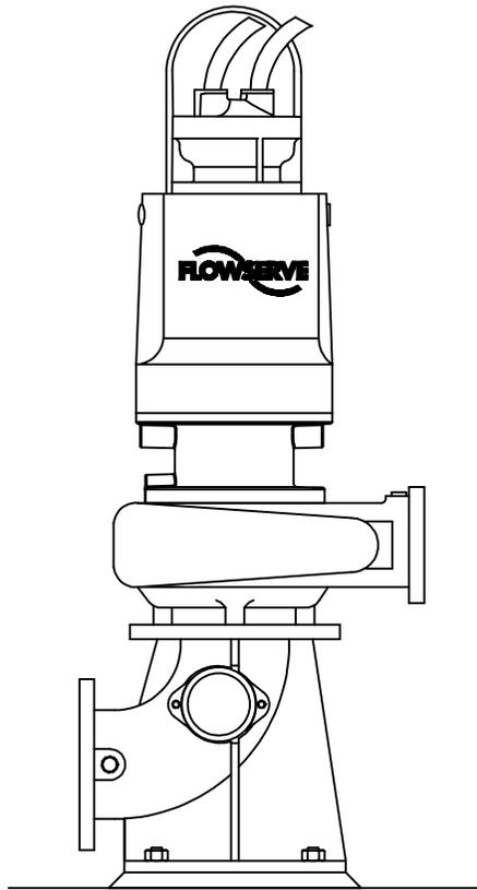
**Figure 2: Dry Pit Installation**
