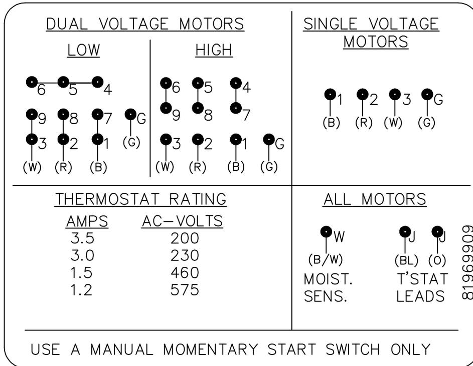
**Figure 5: Motor Connection Diagram**
